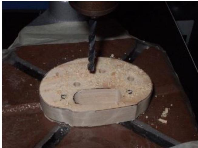
Saw the same shape as the original out of wood. Use a piece of paper (same size) to determine where you will have to drill the holes. Drill them the same way as the original.
