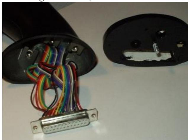
I soldered a new connection . Be sure the hole in the wood is big enough to put the connector through. (in the middle a little wider)
