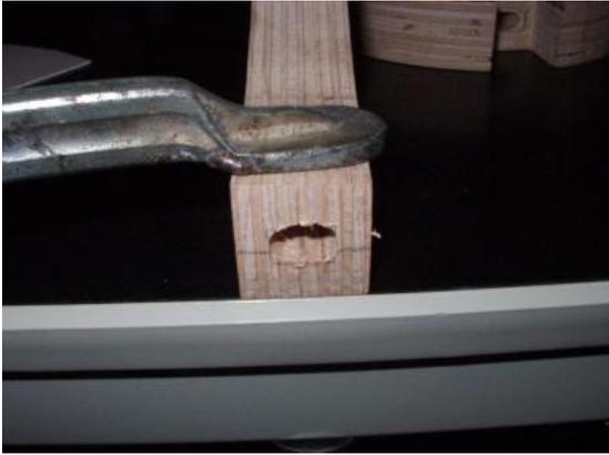
Drill also on both sides a hole in the handle, about 4 cm deep.
