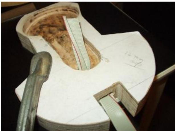
Drill a wide hole in the base of the handle.
