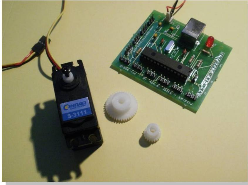
One of the limitations a servo brings with it is the angle of rotation. A normal servo will only rotate over 180 degrees. It is possible to modify the servo so it can rotate over a bigger angle but most of the people will not be eager to open a servo housing and have to cut away some plastic and unsolder the little pot-meter.
