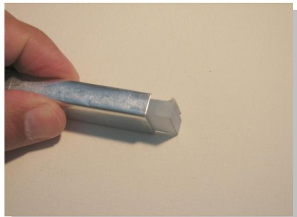
When the pieces are cut make a pair of sticks so it will become easy to bend the pieces at the right distance. Leave the paper on the aluminum until you have bend it, it will be easier to determine the place where to bend.
