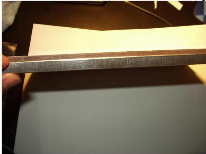
It is a thin display, look at the picture above. I added a 3mm thick plexi glass on top of it. Just used double sided scotch tape for this , it's thin and of a good quality.
