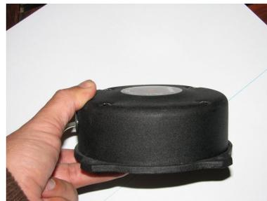
The Shackers have an impedance of 4 OHM or 8 OHM.
