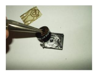
After removing the wheel we can drill some little holes and connect a wire on the spring and another wire on the other side at bottom.
