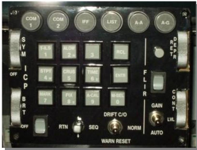
Here I'll try to sketch the way I builded my ICP. As I mentioned earlier in other PDF's and on the site, the panels I made do have the correct measurements but I used not the correct font and especially in case of rotaries I sometimes placed the words a few mm (counter) clockwise, just to match the positions of the 12 step rotaries I used.
