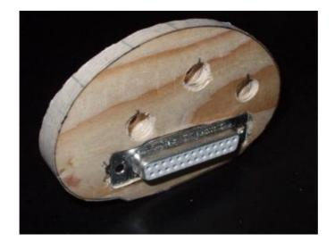
With a knife you can cut 2mm deep at the edge of the tape. Then cut gentle at the backside towards the end of this cut of 2mm deep. In this way you will get a shape that will perfectly fit on the grip.
