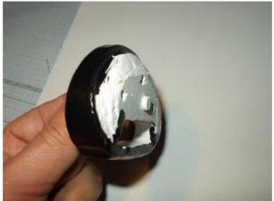
Use the drilled holes on the inside to determine where the wood should be thicker. (here you can see also a bolt through the wood, it is used to fasten it to the wooden-handle)
