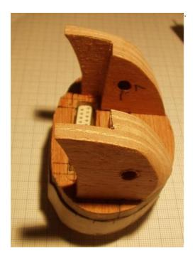
Drill the hole for the bolt. And if all fits, you can screw it together.
