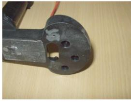
Make the surface of the original flat. Put the cable through the original.
