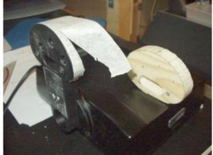
Put on the original some paper tape. Cut of what is over the edge. Hold the new wooden shape beside the original (the flat outside) and draw some lines from the tape on the wood. So you are able to put the tape at the right place on the wood.
