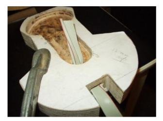
Drill a wide hole in the base of the handle. So a ribbon cable will fit through it. Drill some cm inside the (cougar)throttleshape, there the cable will go into the base.
