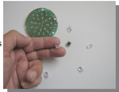
The next step is to solder some wires on the leds. It is handy to use a little clamp to hold the led. In this way the soldering process will be a very quick one so the leds will stay alive.
