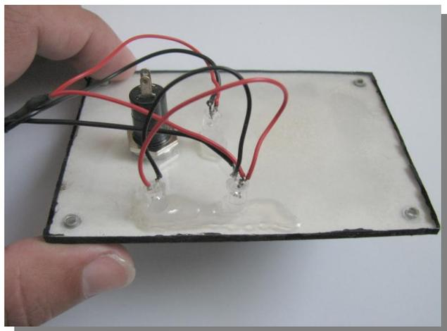
Use a small resistor, when using 5V use 100 OHM or when using 12V use 330 OHM
